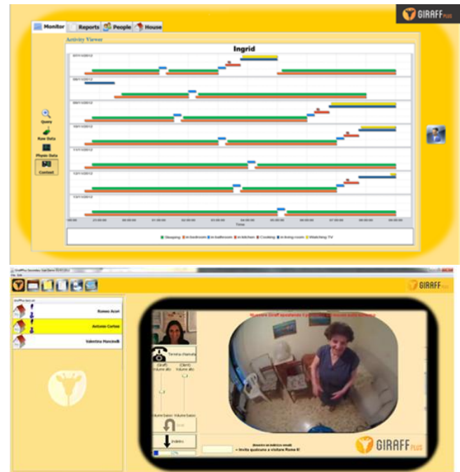
Fig. 5 Upper graph, visualization of night activities: green line - sleeping; orange line – in bedroom; light blue line – in bathroom; light red line – in kitchen; dark red line – cooking; dark blue line – In living room; yellow line – Watching TV. Lower display, interface for the remote driver of the Giraff robot
