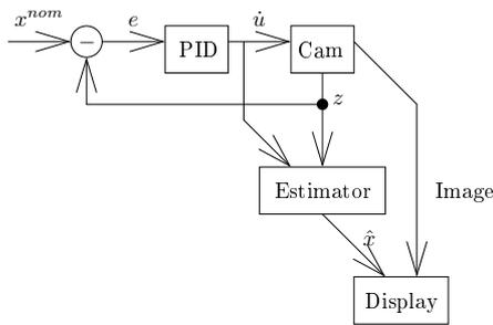
Fig. 4. Camera subsystem of the GroundBot and its user interface in parametric mode.  $x^{nom}$  is the nominal trajectory generated by the active pan/tilt pattern.
