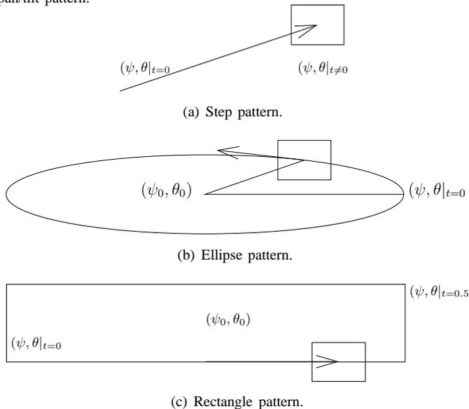
Fig. 5. The selectable parametric pan/tilt patterns.  $t \in [0, 1]$  describes a full period of each pattern. For the step pattern, only a long, first period is used for system tuning.
