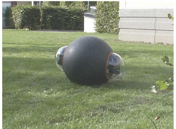
Fig. 1. The spherical security robot GroundBot; a pan/tilt zoom camera is housed in each of the transparent bulbs on either side of the shell.
