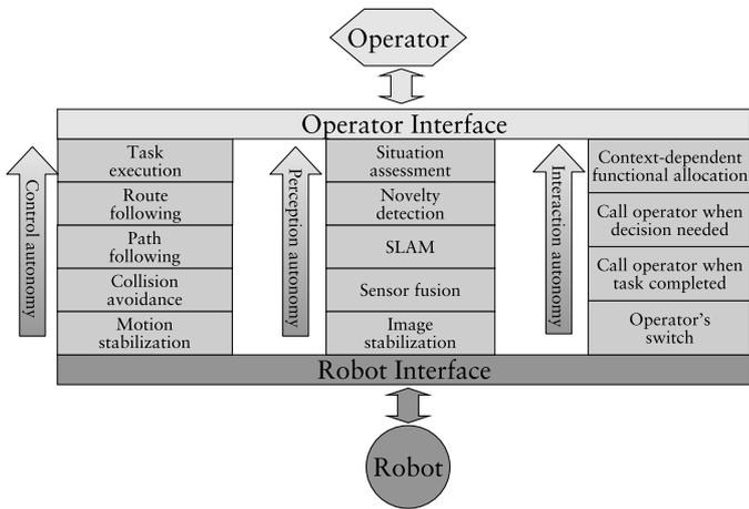
Fig. 2. Illustration of the three towers of autonomy.
