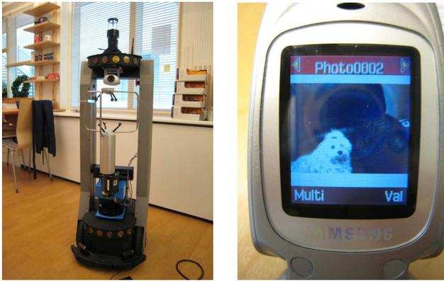
Fig. 5. (Left) Astrid, a mobile robot approaches the living room sofa to take a picture. (Right) The result of the picture taken on the sofa shows that the dog has triggered the pressure sensors.
