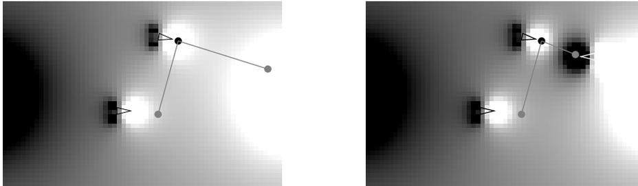
**Fig. 3.** Choosing between the ‘Kick’ and ‘Steal’ behaviors in two different situations. The black dots show the present position of the ball, and the lines and the grey dots, represent the calculated trajectories and predicted final positions (of the ball) respectively when performing the behaviors.
