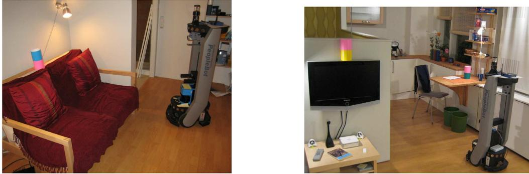
Fig. 2. Two view of the experimental environment. Left: the robot Astrid in the living room facing a sofa. Right: the robot at the entrance of the kitchen. The colored markers used to detect a sofa, a tvset and a table are clearly visible.
