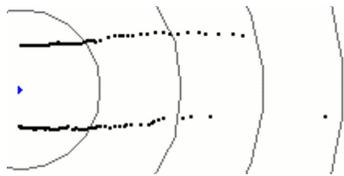
Fig. 7. An example scan from the Tunnel data set. The laser (triangle) is located at the left of the figure facing right. The distance between scale lines is 10 m. Note that readings of maximum range are not displayed.
