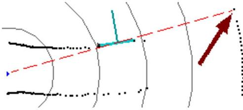
Fig. 12. Example of a scan where the algorithm has falsely detected an opening. The stray range reading causing the false detection is indicated by the arrow. Laser (triangle) to the left of the figure facing right, the distance between the scale lines are 10 m.
