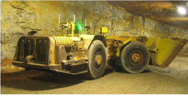
Fig. 1. LHD vehicle prepared with sensors and control system for autonomous navigation.
