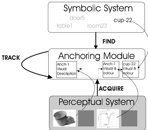
Figure 1: Graphical illustration of the extended anchoring functionalities where bottom-up and top-down information is possible and different sensing modalities are used.
