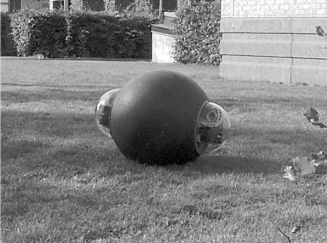
Fig. 2. The spherical security robot GroundBot.
