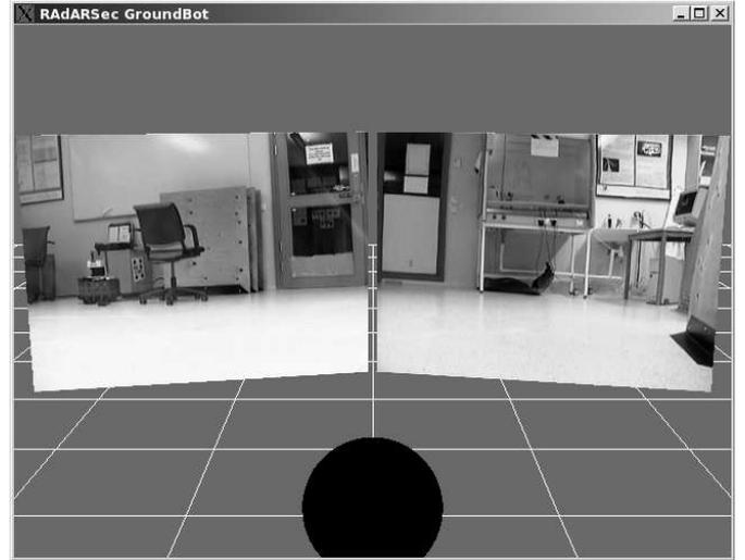
Fig. 4. Screenshot of our graphical user interface in use. The camera position is brought down to a third person view, overlooking the black ball-shaped GroundBot.
