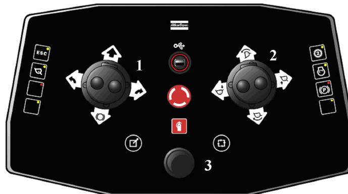
**Figure 3. Operator's station control panel with joysticks (1, 2), jog-dial (3) for menu selection and push buttons for event-based commands**
