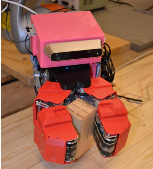
Fig. 1. A power grasp of a wooden object with the Velvet-II dexterous gripper.
