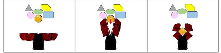
Fig. 2. Grasp Execution Control: (Left) as the gripper starts closing, the current through the opening motor is monitored; (Middle) after the fingertip contact with the object, the actuated belts are switched on to pull it in; (Right) the controller strives to maintain a given current set-point in order to enable compliant in-hand manipulation behavior.
