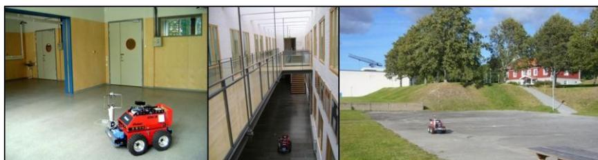
Fig. 2. The prototype pollution monitoring robot during the mission in the experimental environments: an enclosed indoor area (left), a part of a long corridor with open ends and a high ceiling (center), and an outdoor scenario (right).
