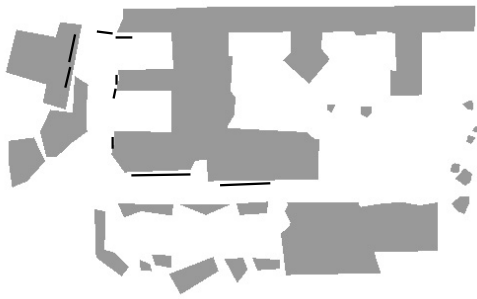
Fig. 2. Occupancy grid map derived from Fig. 3. The wall estimates calculated from the semantic map are drawn in black lines. The semantic map in Fig. 1 belongs to the upper left part of this figure.
