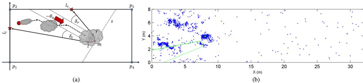
**Figure 1. (a) Construction of the PPE for the micro UAV in real-world environments in non-uniform wind fields. The source location is denoted by the large red dot. (b) PF-based GSL algorithm after 220 iterations using sweeping (blue points = particles and green point = prediction and true gas source location).**
