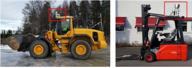
Fig. 7. Wheel loader (left) and forklift (right) on which the camera setup was evaluated. The location of the sensor unit is indicated in red.
