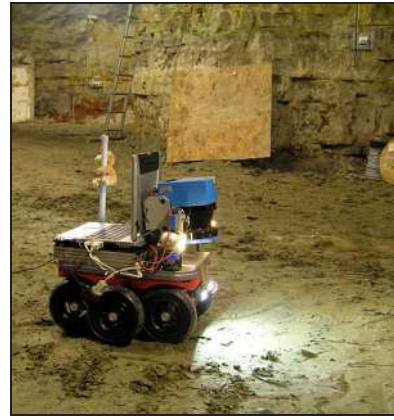
Fig. 3. The Kurt3D robot scanning underground.
