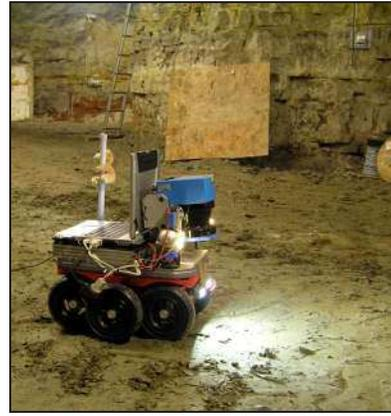
Fig. 3. The Kurt3D robot scanning underground.
