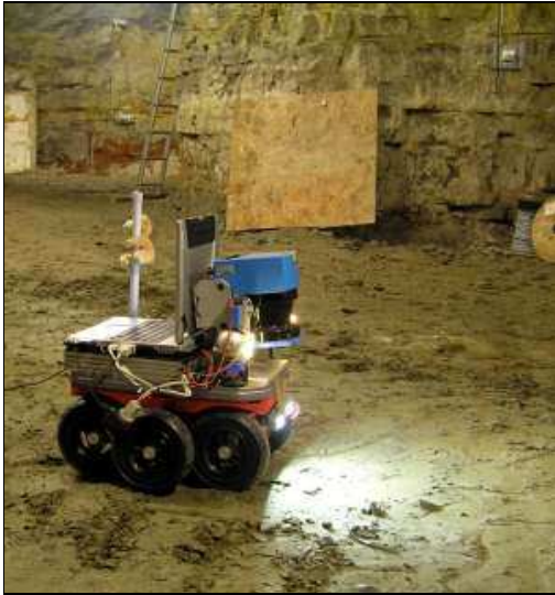
Fig. 3. The Kurt3D robot scanning underground.
