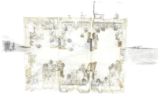
Fig. 7. The reference model created in our evaluation experiment consisting of 3 \times 22 registered scans and the corresponding colours from 7 \times 22 camera images.
