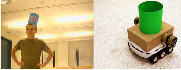
Figure 1: The coloured “hat” that is tracked by the absolute positioning system, worn by a person (left) and placed on a robot (right).
