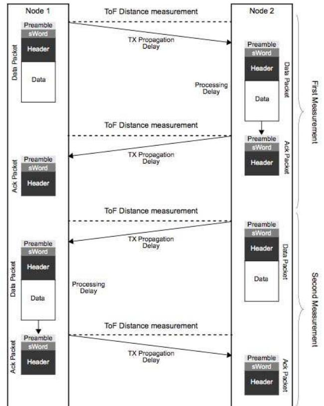
Fig. 1. Symmetrical Double Sided Two Way Ranging Technique
