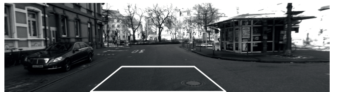
Fig. 2: This figure depicts the region of interest (ROI) in the image that is assumed to be approximately planar.
